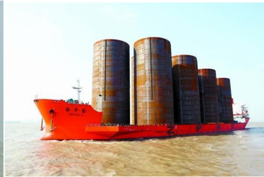
China South Sea Project Diameter:21m Length:85m Weight:705tons/pipe
