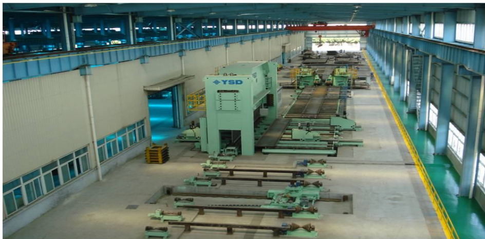
Our International Leading Level JCO lines (for LSAW pipes)
