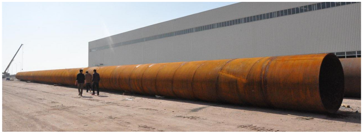
50m Long Pipe Piles lay outside of factory, waiting to be shipped
